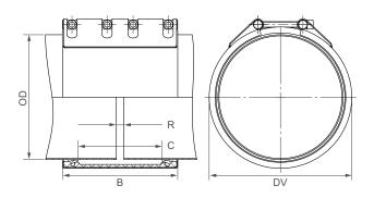
$\begin{array}{ccc} B & \Rightarrow & 310 \text{ up to } 311 \text{ mm} \\ \text{DV} & \Rightarrow & \text{OD} + 38 \text{ mm} \\ \text{C} & \Rightarrow & 227 \text{ mm} \\ \\ \text{R with strip insert} & \Rightarrow 120 \text{ mm} \\ \end{array}$
