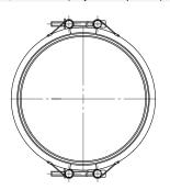
R with strip insert ⇒ 60 mm R without strip insert ⇒ 15 mm
