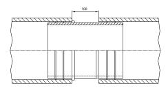
The pipe ends may be centred to each other again and the repair couplers aligned using the notches on the inner coupler. The clamps are to be tightened according to the torque indicated on the label.
