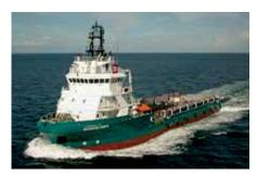
Others: AHT Anchor Handling Tugs, AHTS Anchor Handling Tugs Supply Vessel
