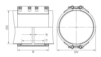
R with strip insert ⇒ 120 mm R without strip insert ⇒ 20 mm
