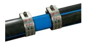
Expose 100 mm of pipe. Slightly bend the pipe ends sideward and insert the repair coupler to the O-Ring into one of the two pipe ends. Align the shells to the pipe ends.
