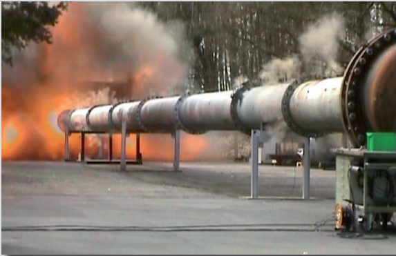
Explosion test with DN 800 / 32" pipe
