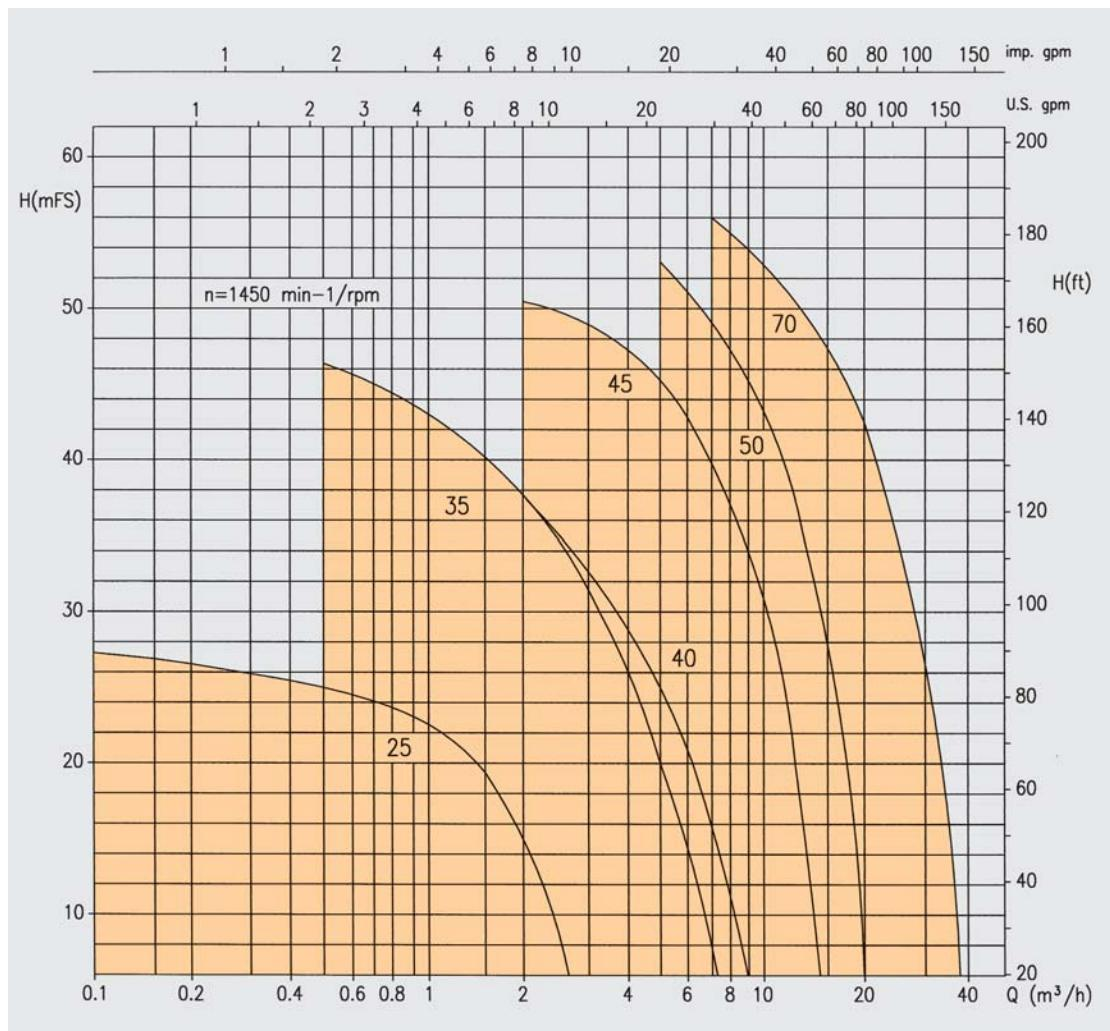
Performance curves of the individual pump sizes, also for 1750 rpm,
