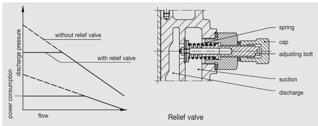
Contrary to centrifugal pumps, the side channel pumps generate a steep head rise and an increased power consumption at lower flow rates. Power consumption and discharge pressure reach the maximum at closed discharge. To protect discharge pipes and to avoid overload of the motors and unacceptable temperature rise in the pump, an additional relief valve can be fitted to the WPV-pumps.
