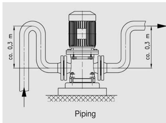
During the suction phase – when priming the empty suction line – the side-channel pumps build up a gas/liquid mixture. The gas or air will be separated and pressed into the pressure pipe while the operating liquid returns to the pump. It is therefore necessary to install the piping in a way that the operating liquid can remain in the pump.
