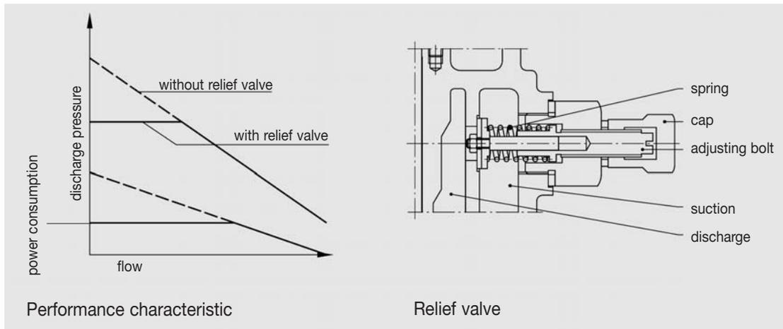
Contrary to centrifugal pumps, the side-channel pumps generate a steep head rise and an increased power consumption at lower flow rates.
