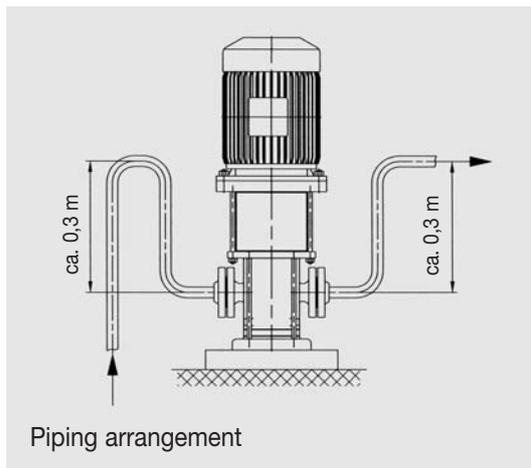
During the suction phase – when priming the empty suction line – the side-channel pumps build up a gas/liquid mixture. The gas or air will be separated and pressed into the pressure pipe while the operating liquid returns to the pump. It is therefore necessary to install the piping in a way that the liquid can remain in the pump.
