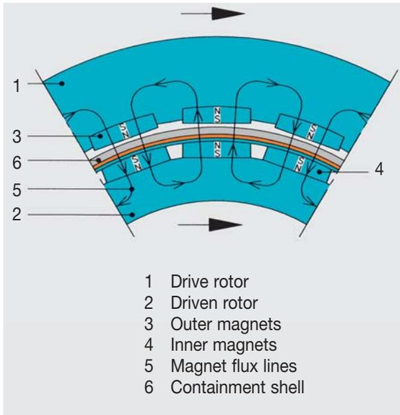
The drive rotor with the drive magnets is keyed to the motor shaft, the driven rotor with the driven magnets is keyed to the pump shaft.
