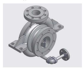
The pump casing forms - together with the containment shell - the pressure retaining pump part. Maximum allowable pressure at PT is determined by the shell design and the material. The pump casing has metal-to-metal fits with confined compression controlled gaskets.
