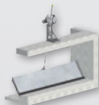
Radial Weir Gate 6.5
