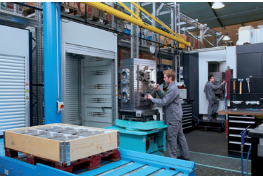
Flexible pallet-based manufacturing system with machining centers
