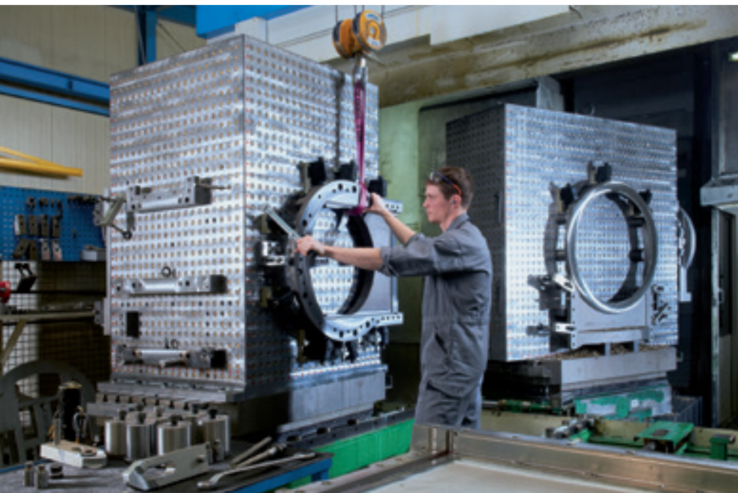
Large valve body milling on horizontal twin table machining center
