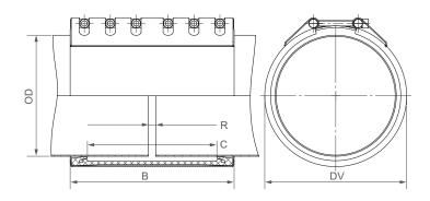
В  $\Rightarrow$ 443 up to 444 mm DV  $\Rightarrow$ OD + 48 mm С  $\Rightarrow$ 350 mm R with strip insert ⇒ 200 mm R without strip insert ⇒ 20 mm
