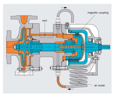
Besides common sealed pumps also sealless pumps with magnetic coupling can be used for hot water. The termination of the main wear part (the mechanical seal) lead to considerably longer "mean time between failure" and therefore higher availability. Hot water spill through seal failure is also excluded. The pump design is self-venting and does not require water cooling. Performance range
