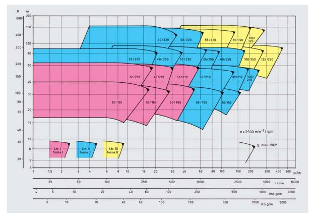
Performance curves for the different pump sizes are available on request, also for 1750 / 3500 rpm.
