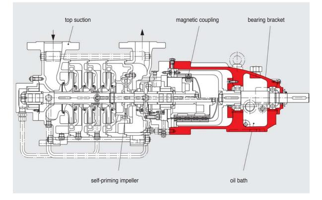
Optional designs – HZSMA, for handling of liquified gases
