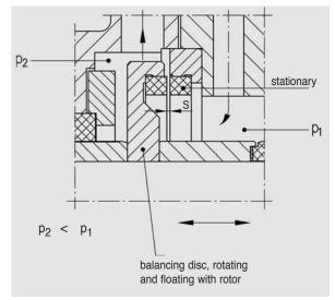
The rear disc side is connected with the pressure side of the first pump stage via an external pipe. According to the rotor position and the adjusting gap S, a counter force is created by the differential pressure between front and rear side of the balancing disc. This counter force acts against the residual load towards the containment shell such that no thrust loads occur. No thrust bearings are required. The start-up rings keep the pump shaft in position during start-up and shut-off.
