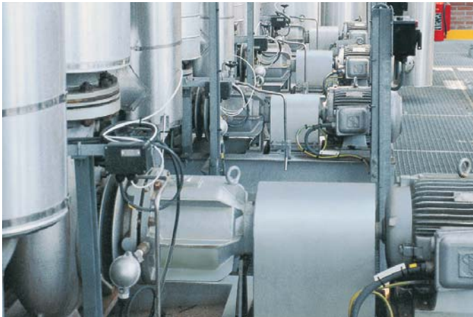
Type NMW with magnetic coupling. Liquid: DOWTHERM-A, 350°C (662°F).
