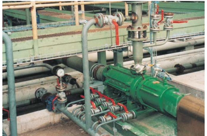
Type HZMR with magnetic coupling. Liquid: Benzol mixture.
