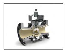
The CeraValve type KSV is a ceramic lined ball valve for On/Off function as well as for Throttling Control applications for corrosive media with abrasive solids content. It is an alternative to PTFE/PFA lined valves in the event that their performance limits (pressure, temperature, wear) are exceeded.
