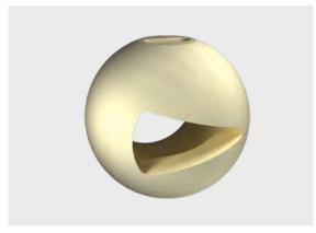
The desired control behaviour of the valve is determined by the nominal diameter of the center housing and the geometry of the ball bore. Round or triangular bores can be rotated by between 0 and 90° and define exact opening cross-sections.
