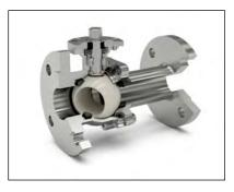
**BR 26 CERA** The valve type BR 26 CERA is a stainless steel ball valve for on/off function with ceramic seats and ceramic ball for service in abrasive and corrosive applications. Especially for abrasive applications in chemical plants this valve can be beneficiary. The basic principle is based on the "floating ball" design. The seats are pushed by o-rings against the ball. This valve can be delivered with a manual handle, with pneumatic- or electric-actuator.
