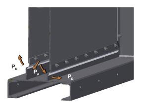
The medium tight shut-off in the duct for such types of dampers is realized by using a seal air system. In such a system seal air is injected between the two blades with relevant pressure, being slightly higher than the pressure of the medium in the duct. Thus a so called "air barrier" is created, giving 100% tightness through the closed damper. It guarantees complete separation of the medium in the duct.
