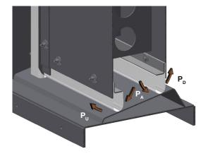
Depending on the application of installation, in which the dampers are mounted, the seal air system can comprise an air preheater. Preheated air protects the dampers from corrosion attack (at defined operating conditions).
